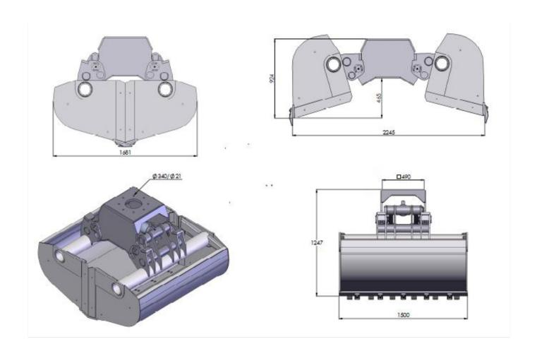
Weight: 1070 kg Volume: 1500 I 32 kN **Gripping force:** Pressure: 250 bar
